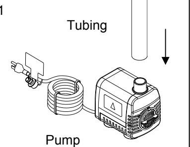
2. Place the pump into the water and connect to a proper power source.
